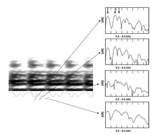
**Figure 1:** Principle of pitch synchronous amplitude adjustment. Left column: signal with pitch marks (bottom) and wide band spectrogram (top). Right column: four wide band spectra. The first three formants are indicated by arrows in the top spectrum.
