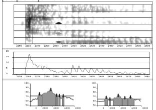
**Figure 2:** Analysis of the original burst for /atu/. Top: wide band spectrogram with the automatic decomposition of the burst into transient and frication noise, Middle: energy contour calculated on a 4 ms window, Bottom: stylized spectra of the transient and noise We will first deal with the quality of the stimuli in gen-
